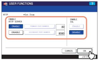
**ENABLE HTTP SERVER** — Press [ENABLE] to enable the HTTP network server service, or [DISABLE] to disable the HTTP network server service. This option must be enabled for using the following functions:
